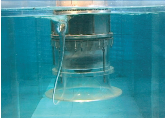
Fig. 105: Laboratory photo of a surface vortex type 6
