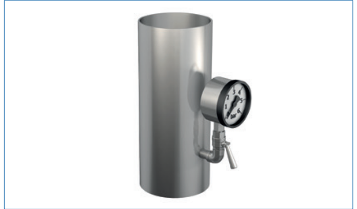
Fig. 79: Pressure measurement in vertical pipe
