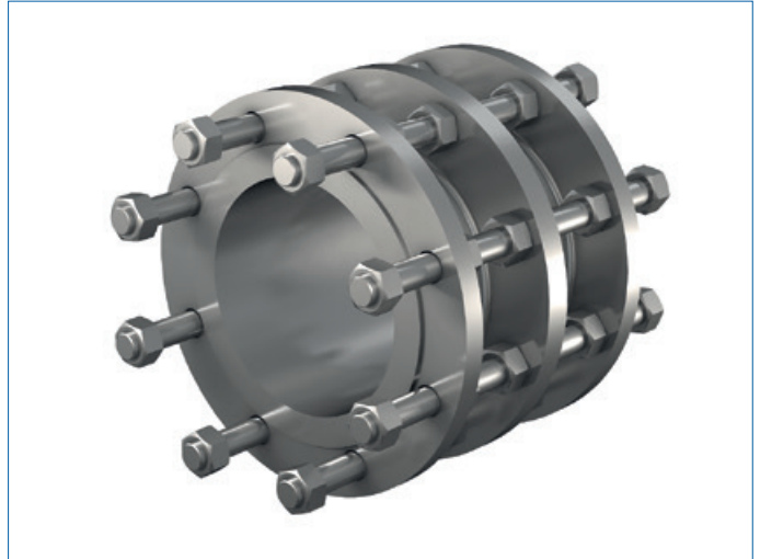
Fig. 80: Expansion and dismantling joint with lockable length adjustment and continuous threaded rods
