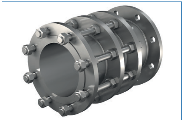
Fig. 81: Expansion and dismantling joint with lockable length adjustment and discontinuous threaded rods
