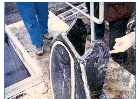
Fig. 3: A DN 800 check valve after surge pressure in the discharge line
