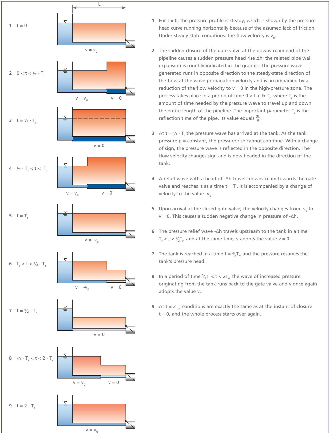
Fig. 8: Pressure and velocity wave development in a single-conduit, frictionless pipeline following its sudden shut-off. Medium shading indicates zones of steady-state pressure, dark shading zones of pressure increase and light shading zones of pressure reduction. The expansion and contraction of the pipeline as a result of rising and falling pressure levels, respectively, are roughly illustrated. To illustrate the extent: If the pressure rises by 100 bar, the volume of water will decrease by about 0.5 %.
