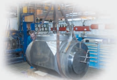
Mounting of line blind valves VTS, DN 600 and DN 800, at KSB works Pegnitz, Germany
