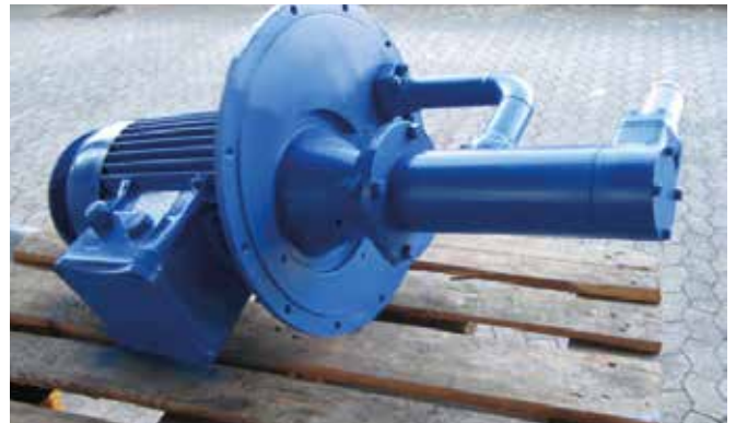
Screw pump – maintenance inspection and commissioning
