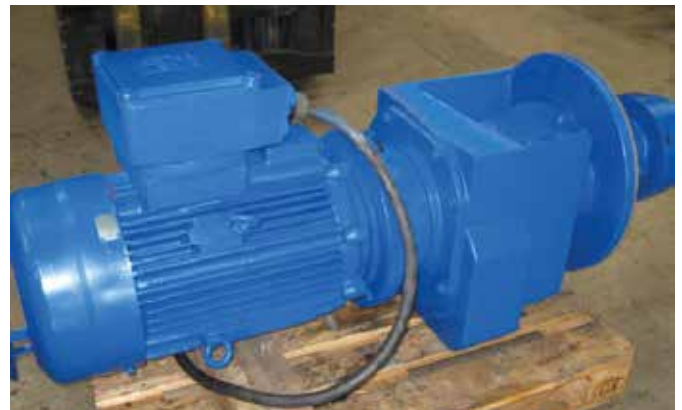
Gear unit including electric motor – maintenance inspection, test run and commissioning
