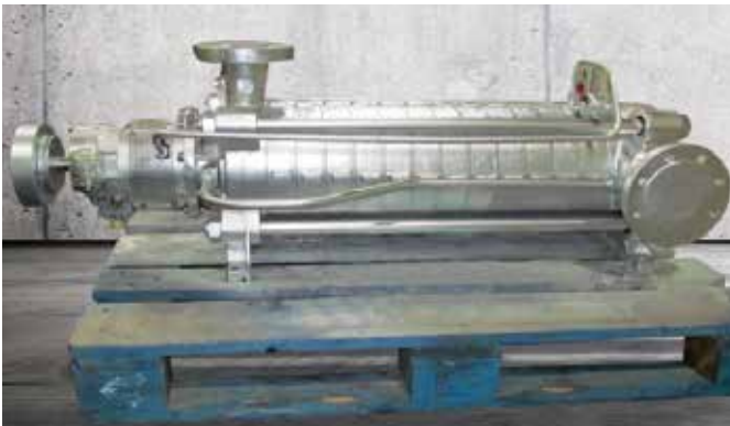
Super-pressure pump – maintenance inspection incl. pressure test, alignment and commissioning
