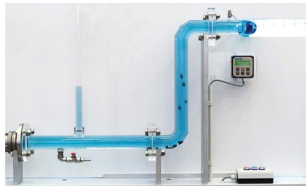
Image 1 shows a test and demonstration model regarding flow velocity. Solids as they may appear in sewage pipes are inside the flexi pipes. The flow velocity is modified by a pump in the back and measured with a flow meter. The flow velocity influences the transport of the solids in the horizontal and vertical pipe. Even if different kind of solids are used, the impact of wipes in the real world would require an even higher minimum flow velocity to transport the composition in the system.
